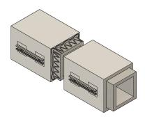
Apply sealant to the interlocking connection
