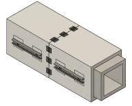
Join the interlocking connection and secure with fasteners
